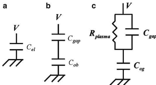
voltage divides across these capacitors proportionally to the inverse of their size. This results in a strong electric field in the gap which can now lead to breakdown and discharge.
