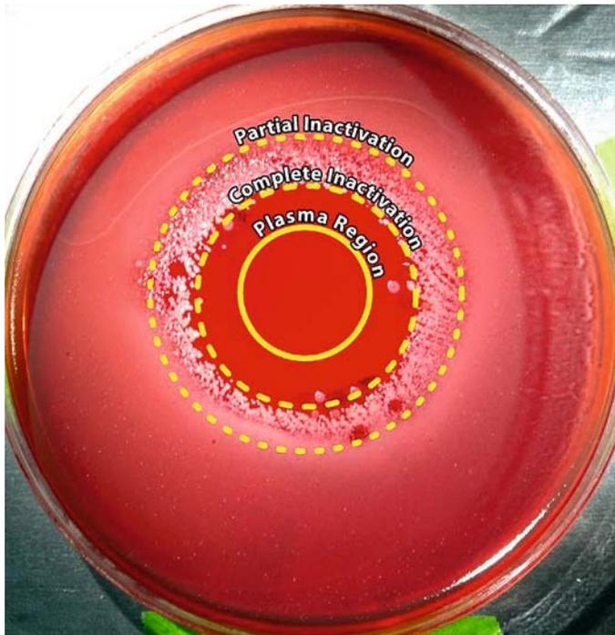
**Fig. 17** Petri dish with blood agar, seeded by  $\sim 1.3 \times 10^7$  cfu/cm<sup>2</sup> ( $10^9$  cfu/ml) of skin flora and then treated by FE-DBD plasma for 10 s. While the plasma region diameter is roughly 25 mm, the “inner” circle of inactivated bacteria and fungi diameter is  $\sim 35$  mm and the “outer” circle where the bacteria is partially inactivated (colonies are visible) is  $\sim 54$  mm
